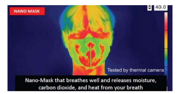
Material: Polypropylene Spun-Bond Non-woven Fabrics, plastic coated wire, Polypropylene loop, nylon string
